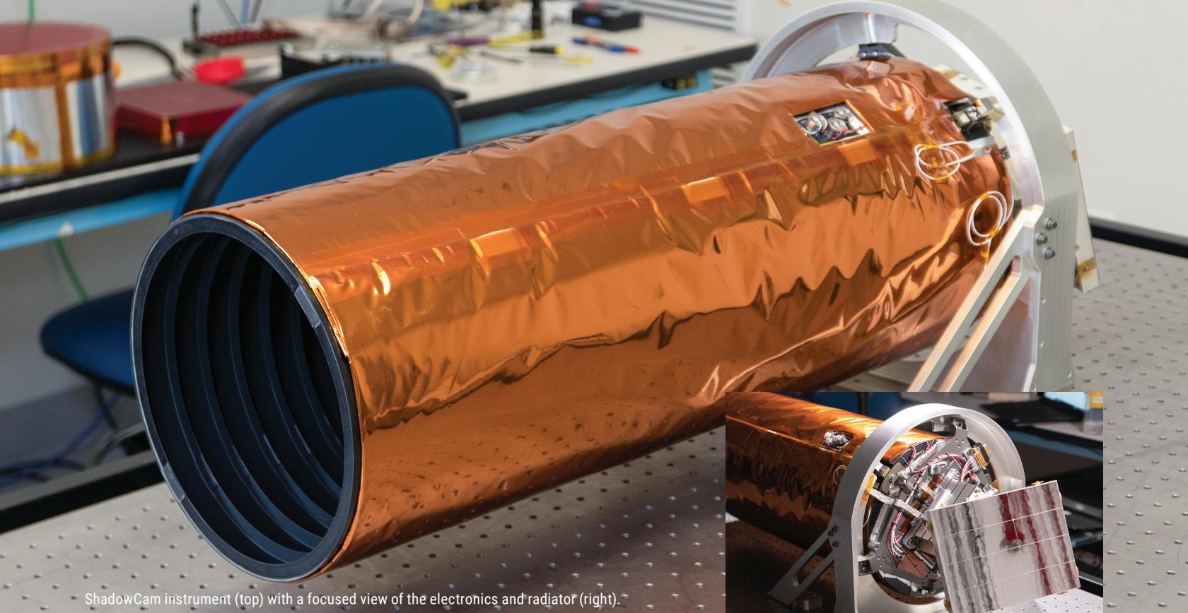
ShadowCam instrument (top) with a focused view of the electronics and radiator (right).
